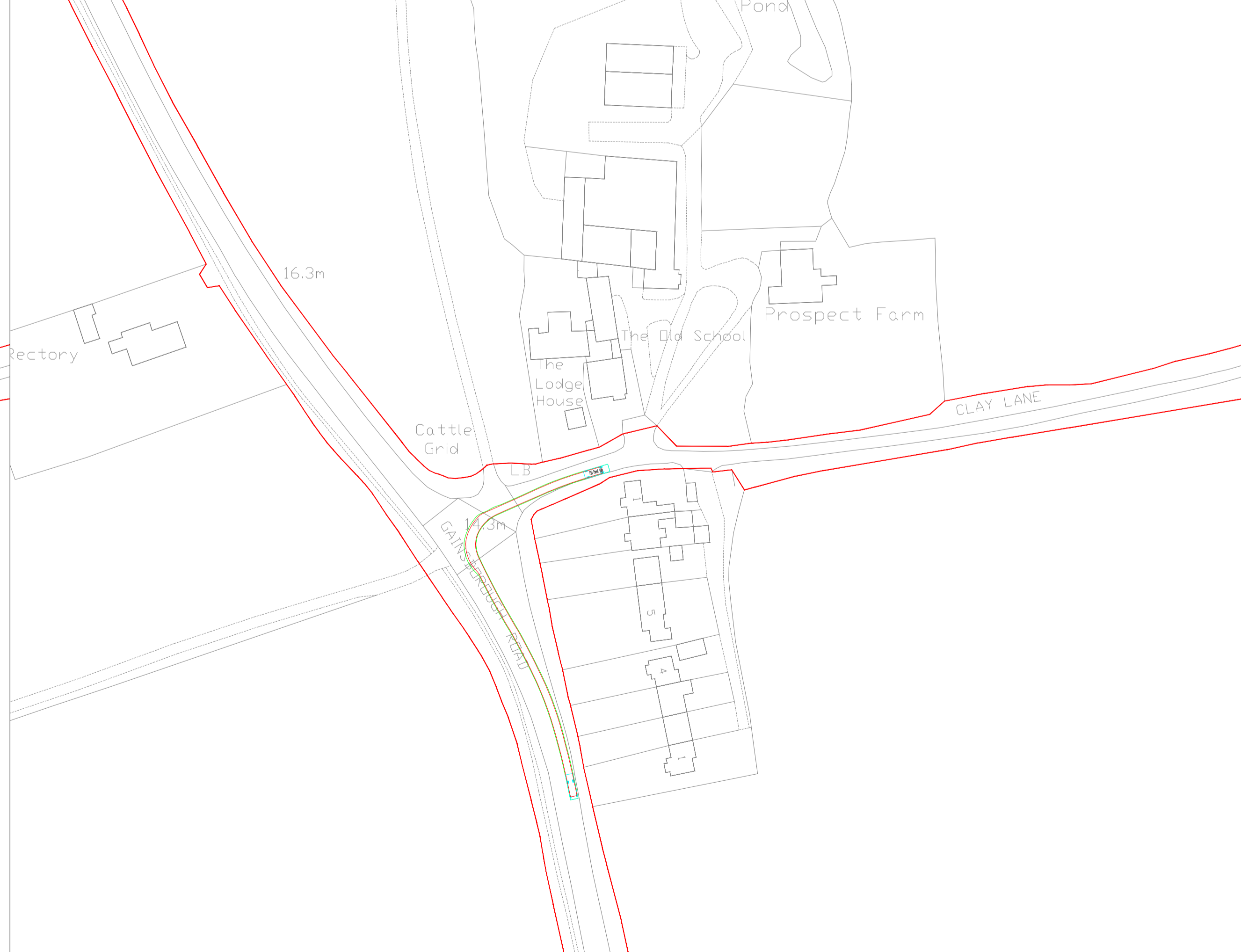
7.5t PANEL VAN VEHICLE MANOUVRE, HEADING WEST OUT OF CLAY LANE TURNING LEFT ONTO ON GAINSBOROUGH ROAD A156 HEADING SOUTH - SCALE 1:1000
