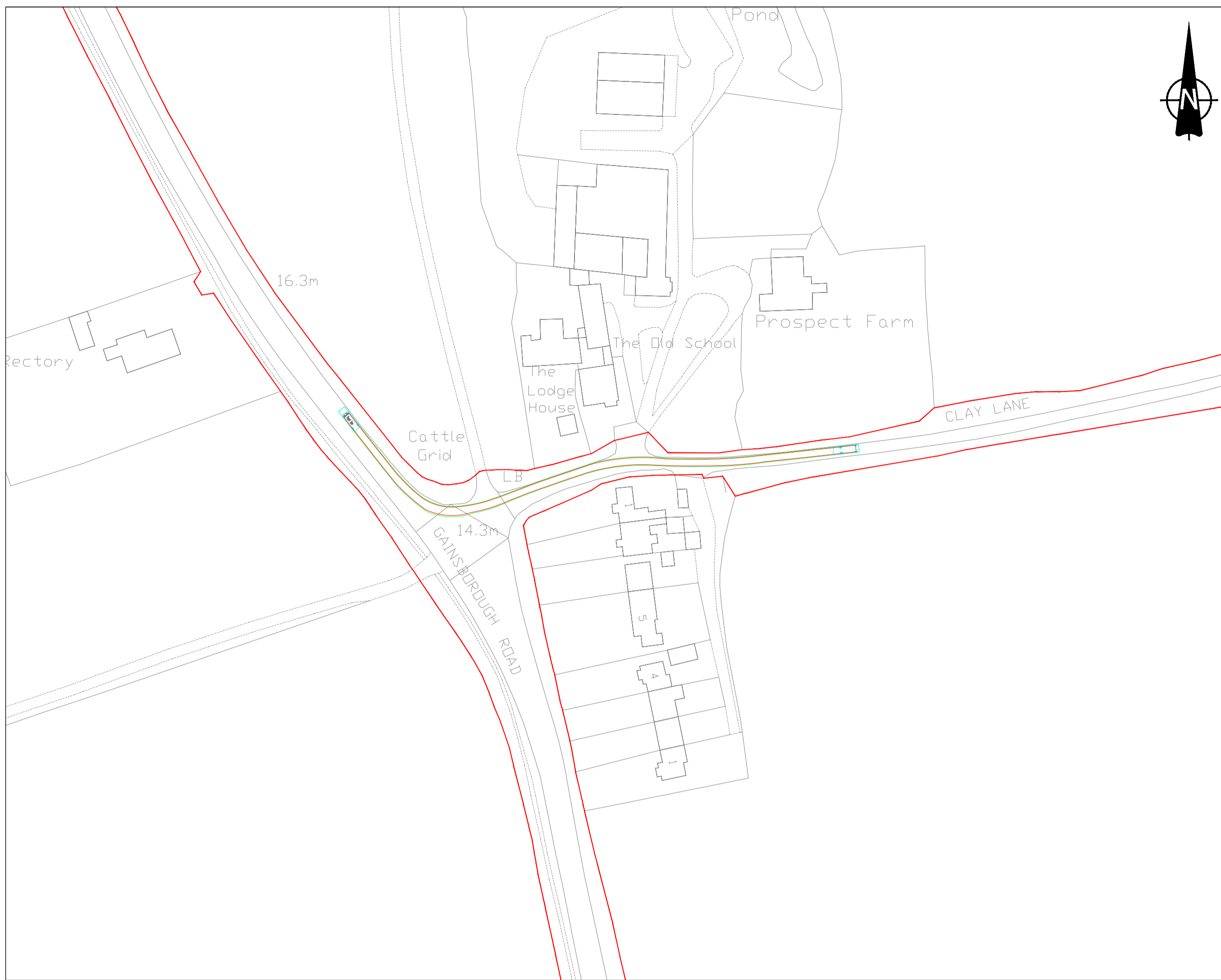
7.5t PANEL VAN VEHICLE MANOUVRE, HEADING SOUTH ON GAINSBOROUGH ROAD A156 TURNING LEFT INTO CLAY LANE HEADING EAST - SCALE 1:1000
